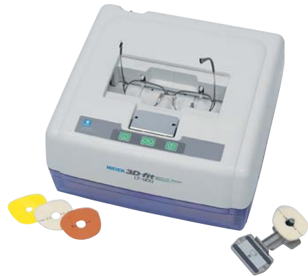
LT-1000 3D satellite tracer with color LCD touch panel and shape editor
